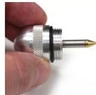
**5** REMOVE the puncture object if there is one, and note the object's angle in the tire tread before inserting the plug. USE **Air Stopper** in the hole to temporarily keep air from escaping.
